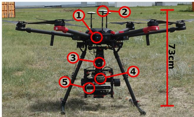
Fig. 1. The experimental setup for VT&R on our multirotor UAV: (1) DJI Matrice 600 Pro vehicle platform, (2) DJI A3 triple-redundant GPS module, (3) DJI Ronin-MX 3-axis gimbal, (4) NVIDIA Tegra TX2, (5) StereoLabs ZED camera.
